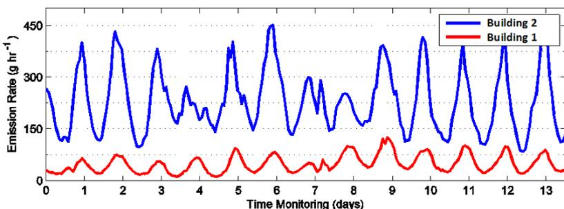
Fig 2. The emission rate of ammonia (g per hour) from both buildings over the monitoring period
