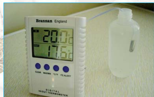
Measure the temperature of liquid and not air.
