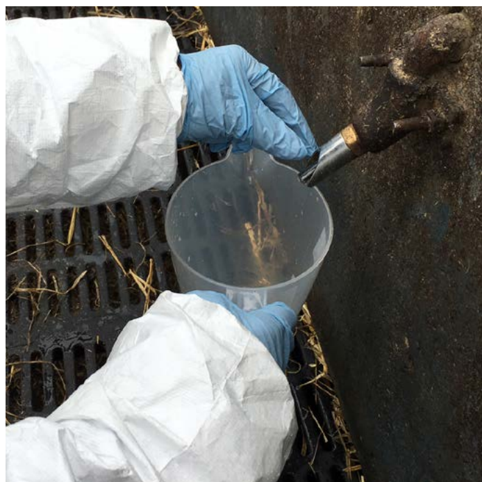
Figure 4. Measuring water flow rate
