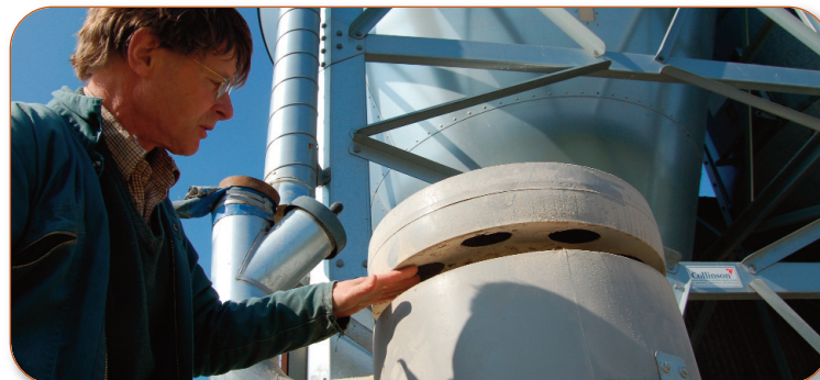
The cyclone attaches to the exhaust pipe on feed bins to collect dust
